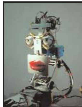
Roboreceptionist: Inkha, who does not just react to people but interacts, runs off a standard PC
