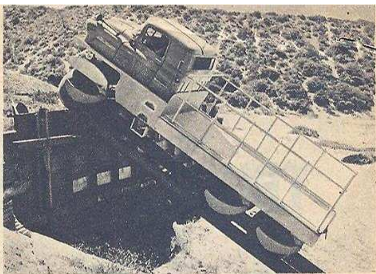
POLE CLIMBING truck goes like a lynx up smooth logs at a 70 per cent incline.
