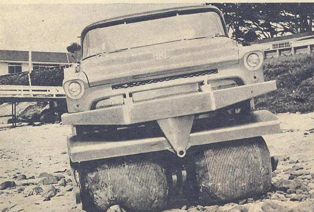
GREAT BIG STONES break no bones, make no obstacles for Rolligon's airbags.
