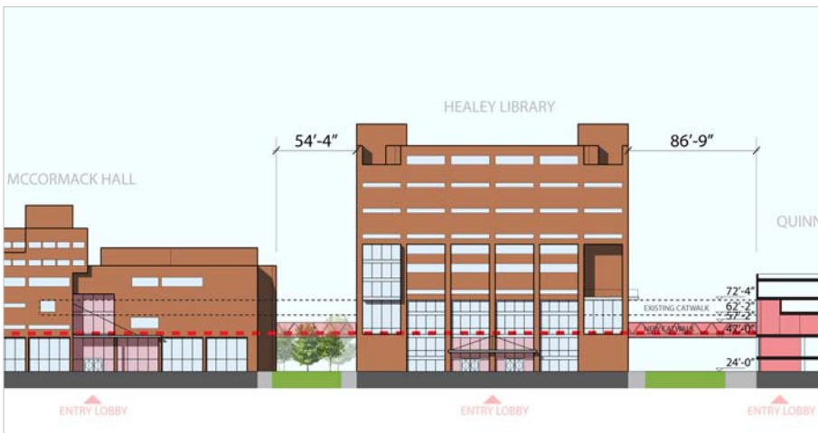
Alternative west (Quad) elevation of Healey Library and new facade to its exposed lower floors after the Substructure's demolition
