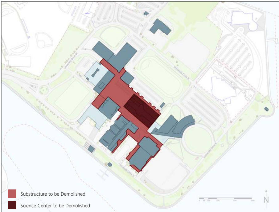
Proposed demolition related to Substructure
