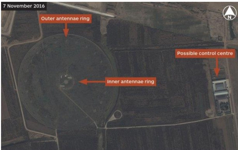
Airbus Defence and Space imagery showing a Circularly Disposed Antenna Array (CDA) site south of Beijing, China. The site was constructed between 2006 and 2010. Sites such as this are used for radio direction finding. Although this capability is primarily used by military intelligence, it can be a useful input for foreign intelligence agencies seeking to corroborate information from other sources.
