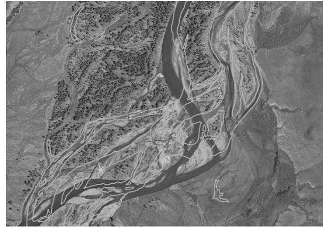
Instability of a gravel bed braided channel
