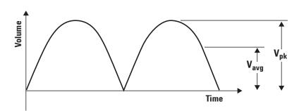
Figure 2.  $V_{ava}$  is calculated based on the absolute value of the waveform.
