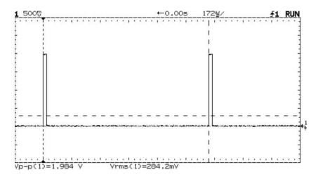
Figure 5. Measuring rms on a low-duty-cycle pulse train
