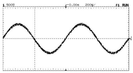
Figure 6. Measuring rms on a noisy sine wave
