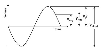
Figure 1. Common voltage parameters
