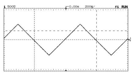
Figure 4. Measuring rms on a triangle wave
