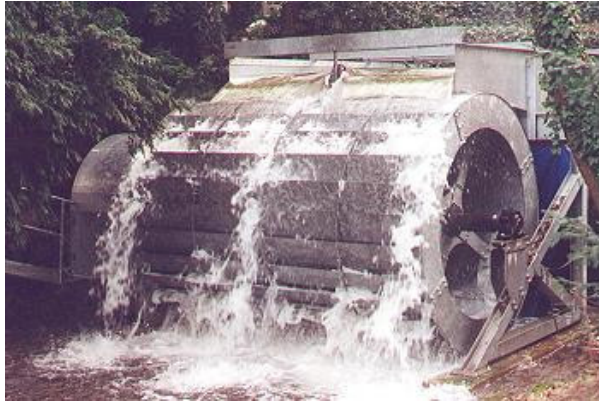
a. 26 kW (el.) overshoot wheel, Freiburg/Germany, 2.9m dia., 4m width (2000) b. New Zuppinger wheel, 6.5m dia., 20 kW (el.) (1996)
