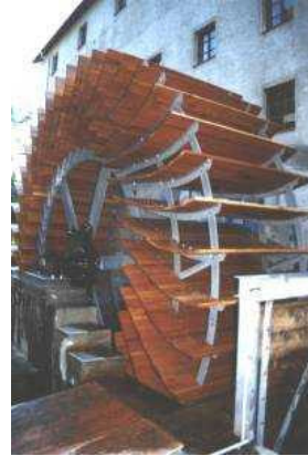
a. 26 kW (el.) overshoot wheel, Freiburg/Germany, 2.9m dia., 4m width (2000) b. New Zuppinger wheel, 6.5m dia., 20 kW (el.) (1996)
