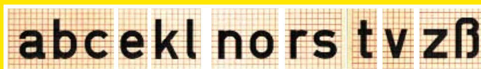
DIN 1451 'Mittelschrift' for hand lettering, preliminary version from 1931
