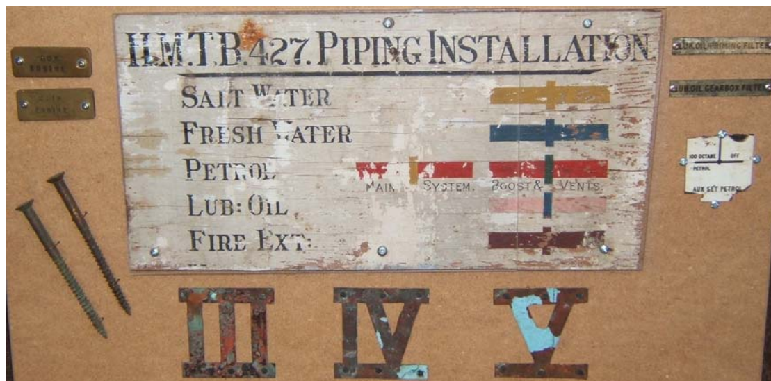
The remains of S-8: Engine room 'Piping Installation' plate, draught marks and brass and plastic identification plates. (Photo: Tim Deacon)
