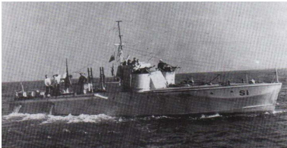
Polish MGB S-1, 'Chart', ('Greyhound'), originally designed for use with torpedoes (note the 'scalloped' sheer line), but used as a MGB
