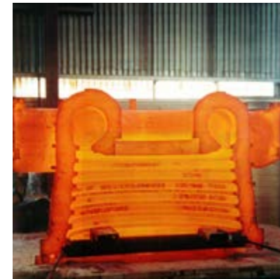
Top: Bottom half of the casing on the treatment hearth at Transtec Engineering Hillside.
