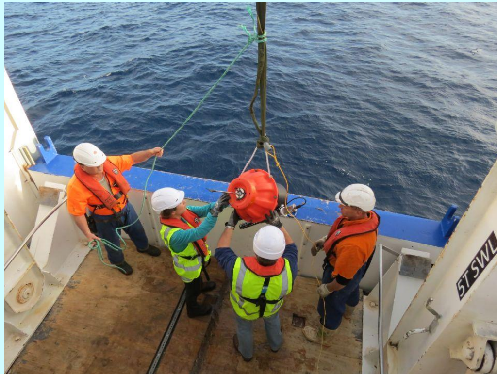
Deep SOLO Float deployment, R/V Tangaroa June 2014, south-west Pacific
