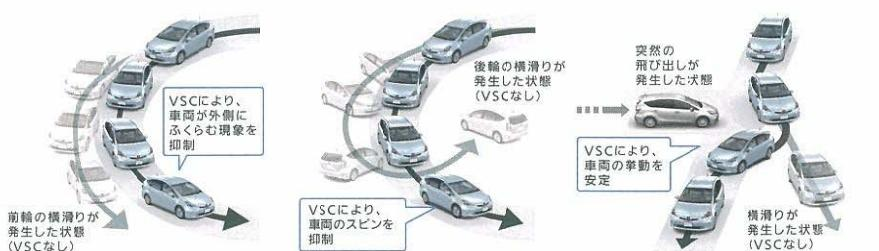
\*1.S-VSC:Steering-assisted Vehicle Stability Control \*2.TRC:Traction Control
