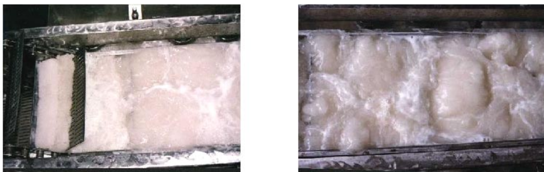
Figure 9.5. HyFloFreeze ® prototype: hydrofluidized bed of highly turbulent ice slurry (Fikiin, 2003).
