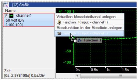
Figure 4-16: Creating a measurement function in the measurement list using drag & drop
