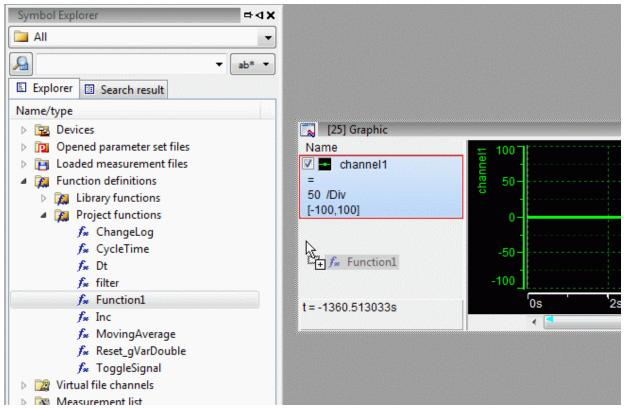
Figure 4-3: Moving the function from the Symbol Explorer to a Graphic window
