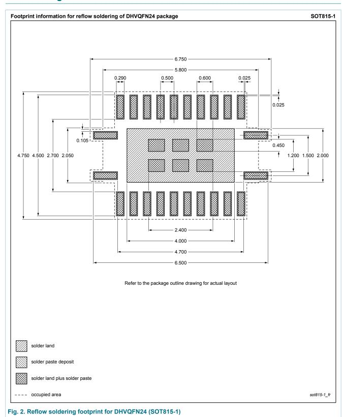
plastic dual in-line compatible thermal enhanced very thin quad flat package; no leads; 24 terminals; body 3.5 x 5.5 x 0.85 mm
