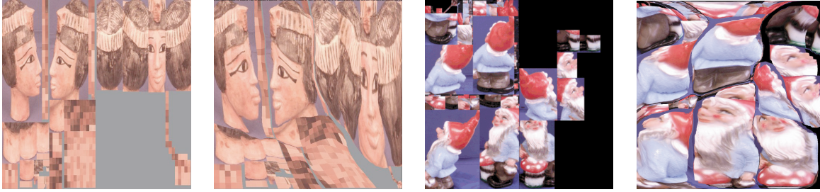
Figure 7: Results of the relaxation algorithm applied to two different texture images. Note how background pixels are reduced to a very small area in the final optimized image. Also, areas of the images with high frequency content are expanded relatively more than regions with smooth color variations. The warping preserves continuity and smoothness in the image. The updated texture coordinates undo the warping. A traditional texturing pipeline can be used with these images (see also Color Plates.)
