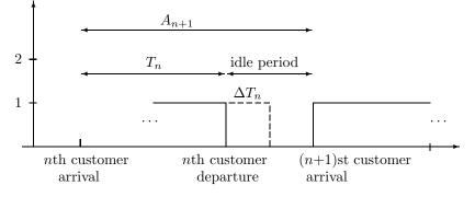
Figure 1: Quantities used in deriving FCFS single-server queue SPA estimator.
