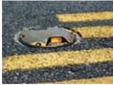
In-Pavement Runway Guard Light
