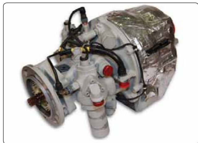
Figure 12-5. Hydraulic power pack.
