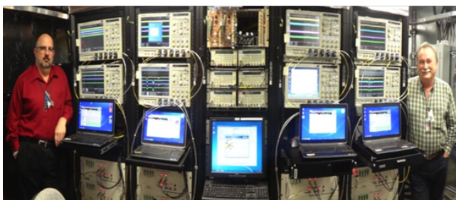
Figure 2. Multiplexed velocimetry system to capture over 100 data channels per experiment.
