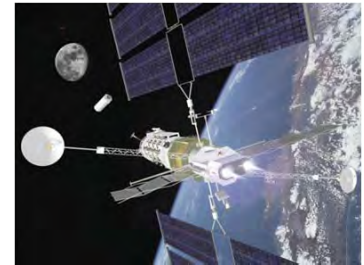
Artist's conception of 200 kW VASIMR Solar Electric Propulsion (SEP) Vehicle.
