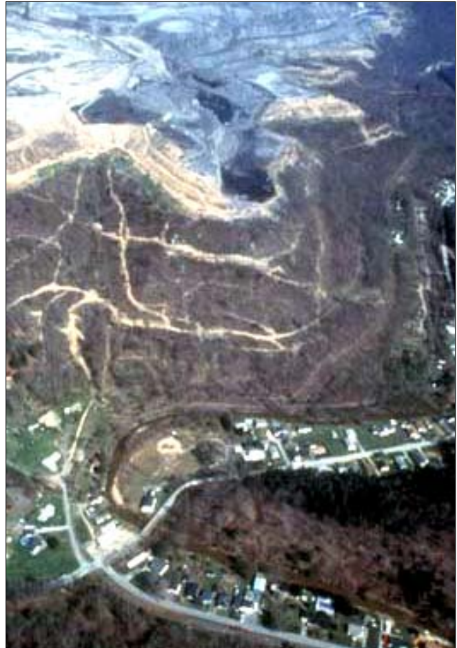
Fig. 1. Large mountaintop removal mines loom over small communities, predisposing them to devastating floods. Valley fill permits authorize the waste from mines to be disposed of in headwater streams. (Photo from www.appalachian-center.org )
