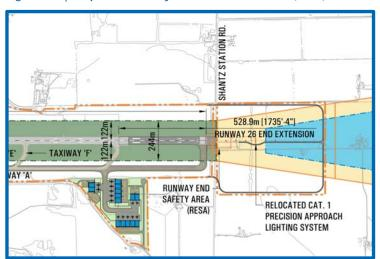
Figure D-2 | Proposed Runway 08-26 Extension Plan (inset)
