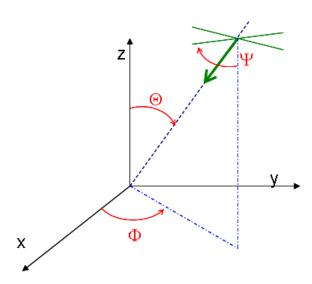
Figure 2.4: Relationship between TT wave frame and detector frame. For an interferometer, the arms are located at the x, y-axis. The angle  $(\theta, \phi, \psi)$  are the Euler Angle of the transformation between detector frame and wave frame.
