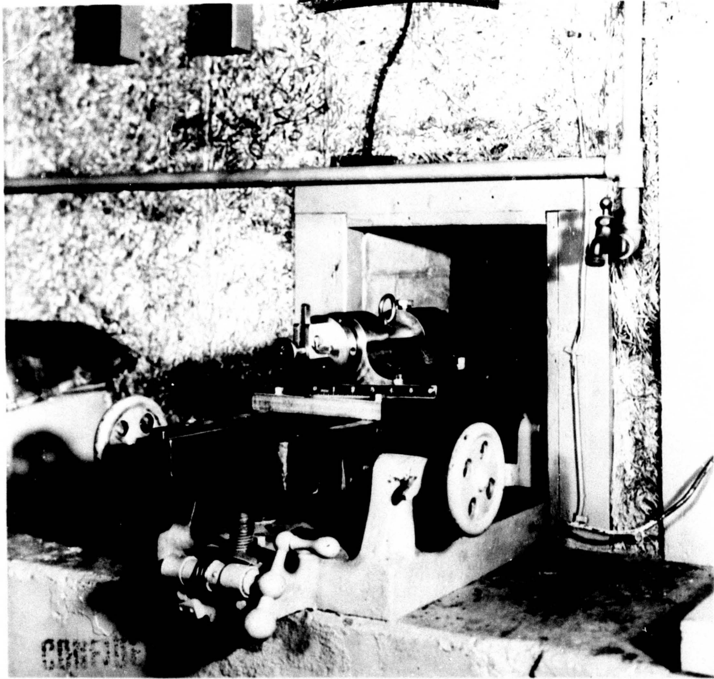
A61275 [REDACTED] & ABERDEEN PROVING GROUND 15 April 1950 Project No. TS2-2015. 9th Report. Ordnance Factory Pressure Housing: Caliber .280 Barrel Fitted to Housing. Note adaption of housing to FA Rest.
