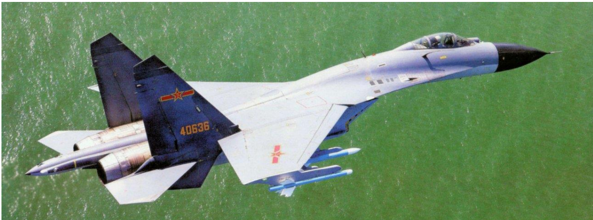
The Shenyang Aircraft Corporation J-11, a Chinese version of Russia's Sukhoi Su-27 'Flanker' fighter series, is regarded as a prime example of Chinese reverse engineering. (Source unknown) 1647627
