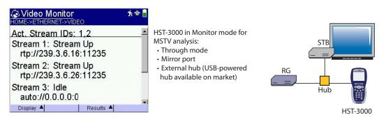
Figure 3. HST Video Monitor screen with active streams present
