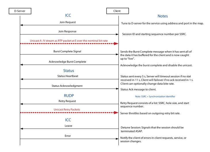
Figure 4. Message flows between the Mediaroom client and the STB
