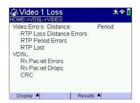
The next analysis screen combines the correlation between RTP packet analysis and the physical layer of the test access point.
