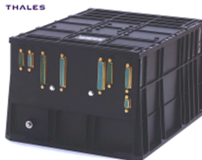
Figure 10 : SARAL ARGOS-3 reception instrument
