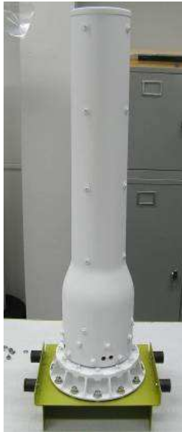
Figure 9 : SARAL UHF antenna
