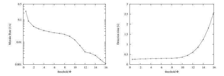
Fig. 8. Exp. 1: average mistake rate as a function of threshold  $\Phi$ . Fig. 9. Exp 2: average detection time as a function of threshold  $\Phi$ . Vertical axis is logarithmic.
