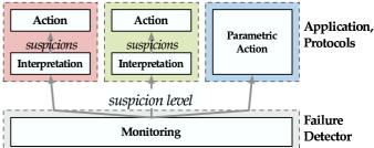
Fig. 2. Structure of traditional failure detectors. Monitoring and interpretation are combined. Interactions with applications and protocols is boolean.
