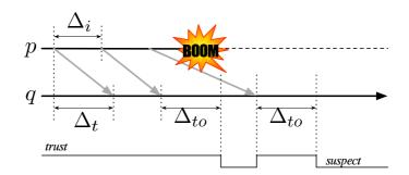
Fig. 1. Heartbeat failure detection and its main parameters.
