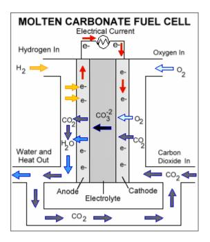
$(\text{LiAlO}_2)$  matrix. Since they operate at extremely high temperatures of 650°C (roughly 1,200°F) and above, non-precious metals can be used as catalysts at the anode and cathode, reducing costs.
