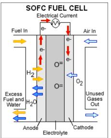
electrolyte is a solid, the cells do not have to be constructed in the plate-like configuration typical of other fuel cell types. SOFCs are expected to be around 50-60 percent efficient at converting fuel to electricity. In applications designed to capture and utilize the system's waste heat (co-generation), overall fuel use efficiencies could top 80-85 percent.
