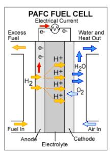
PAFCs are more tolerant of impurities in the reformate than PEM cells, which are easily "poisoned" by carbon monoxide—carbon monoxide binds to the platinum catalyst at the anode, decreasing the fuel cell's efficiency. They are
