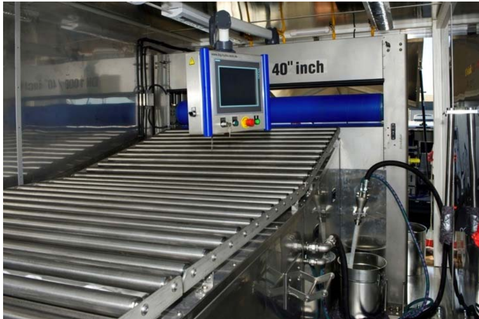
Computer controlled mixing and impregnation equipment
