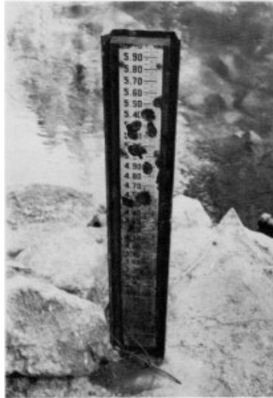
Illustration 53. Staff water gauge at Pohono Bridge. Photo by Robert C. Pavlik, 1985.
