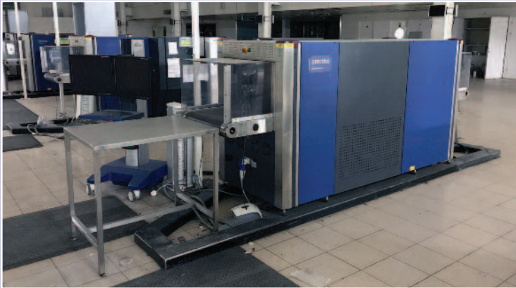
(12) Smiths Heimann Baggage Scanners, HI-SCAN 6040 aTiX and HI-SCAN 6046si
