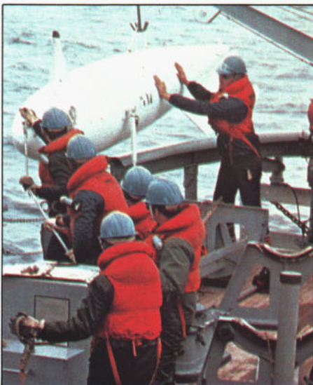
USS Implicit (MSO 455) transits Alaskan coastline during early morning. All hands on USS Constant (MSO 427) participate during minesweeping operations: (top left) crew members maneuver electrical cables; (left) a 900-pound buoy, attached to a minesweeping cable, is hoisted aboard. Reserve SN Ken Reed (above) readies a mooring line. USS Gallant (MSO 489) pulls into Ketchikan, Alaska.
