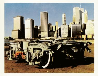
ary suspension which is a combination of steel coil springs and rubber springs. The suspension system does not contain parts which are subject to wear and tear and is easily maintained.
