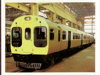
Since 1981, on the order of the New Zealand Railway, GANZ-MAVAG has been supplying 44 electric multiple-unit trains, as commuter trains for Wellington. The propulsion equipment is manufactured by the British General Electric Company (GEC) and assembled by GANZ-MAVAG. The trains are provided with cam control.
