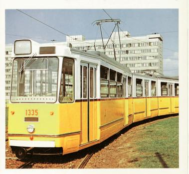
As many as 200 vehicles of this type, introduced by GANZ-MAVAG 14 years ago, have been procured for the Budapest Transit Authority. The cars are of all electric type and of high reliability feature. The efficiency of the articulated light rail vehicle is represented by the fact that a train of two remote controlled articulated cars with one driver can take as many as 524 passengers.
