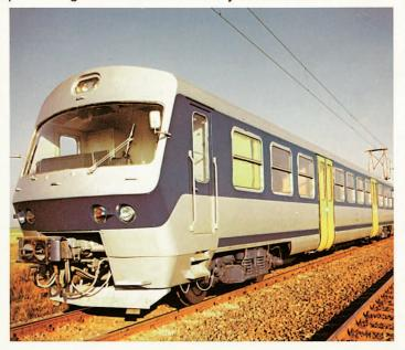
The three-car electric train set consists of two trailers with driver's cab and a motor car in the middle. Two or three sets can be connected into one train by means of automatic couplers so that 6 or 9 cars can run together.
