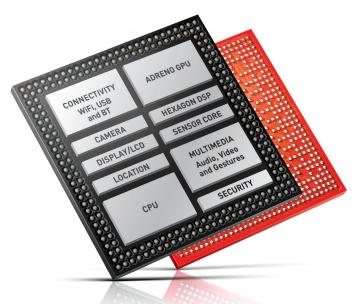
The Snapdragon 600 processor is designed to run 1080p HD video, handle up to 20MP images and render intensive 3D on dedicated components, freeing the quad-core Krait CPU for the main embedded application.
