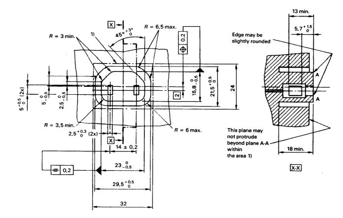
The sketches are not intended to govern design except as regards the dimensions shown. For the symbols indicating the tolerance of form and of position, see ISO 1101.
