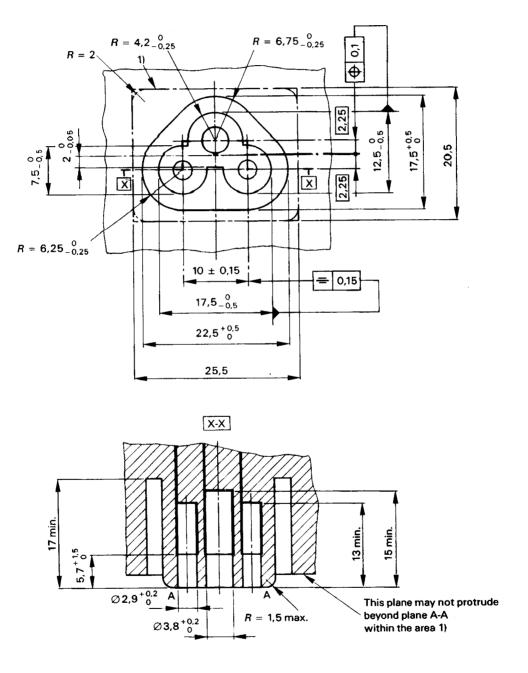
The sketches are not intended to govern design except as regards the dimensions shown. For the symbols indicating the tolerance of form and of position, see ISO 1101.
