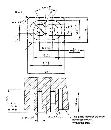
The sketches are not intended to govern design except as regards the dimensions shown. For the symbols indicating the tolerance of form and of position, see ISO 1101.
