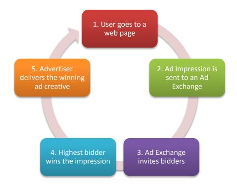
Figure 1: Real Time Bidding Process
