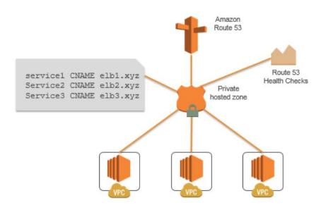
Figure 9: Domain Name System-based service discovery
