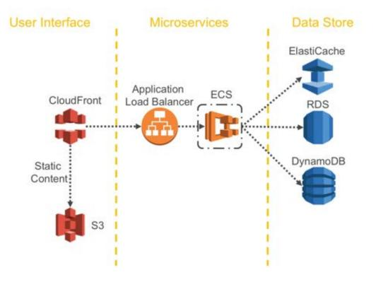
Figure 4: Typical microservices application on AWS
