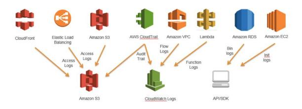
Figure 17: Logging capabilities of AWS services
