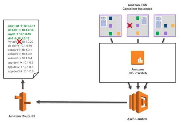
Figure 10: Service discovery using Amazon ECS event stream
