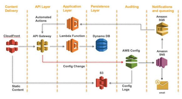
Figure 23: Detecting security violations with AWS Config
