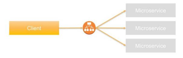
Figure 8: Application Load Balancer-based service discovery
