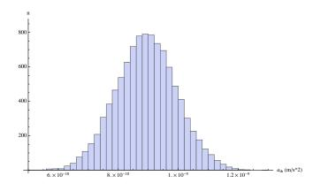
FIG. 6. Histogram for the distribution resulting from the Monte Carlo simulation with 10000 iterations for the thermal acceleration of the spacecraft at t = 8 years after launch.
