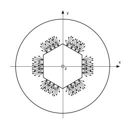
FIG. 3. Schematics of the configuration of Lambertian sources used to model the lateral walls of the main equipment compartment.
