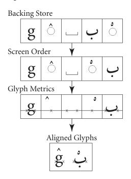
Figure 5-9. Bidirectional Placement
