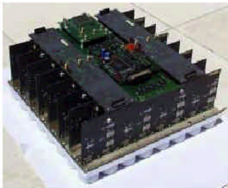
Figure 1 - CEA-FAR Antenna Tile (Exposed Rear View)
