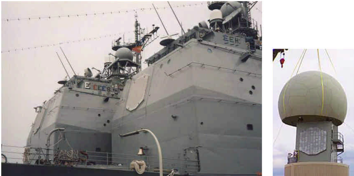
Figure F-2. AN/SPY-1A onboard the Ticonderoga and during installation at the NSSL.
