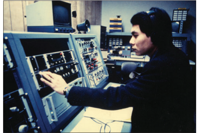
Figure 19: In this 1986 image, a DS Security Engineering Officer adjusts the settings of a CEI VHF receiver (left) and uses a Drake MSR-FM receiver (far right, under speaker horn). The two receivers monitor radio signals from unauthorized sources at a Department of State facility. The monitoring systems were the last generation of vacuum-tube receivers used by DS. Source: Bureau of Diplomatic Security Files.
