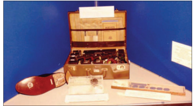
Figure 20: The Shoe Bug (at left). The shoe has the heel removed to show where the bug was hidden. SY officer Lou Grob was monitoring a secure acoustic conference room and discovered the bug in a Foreign Service Officer’s shoe. Source: Department of State.
