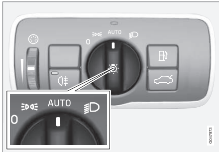
Headlight switch in the AUTO position
