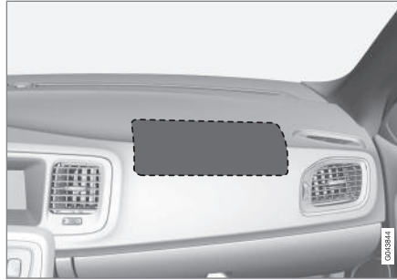
Location of the passenger's side front airbag
