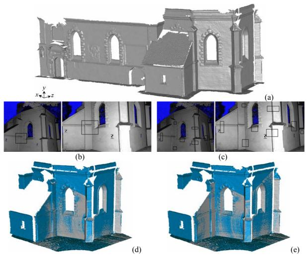
Fig. 9. Example "Wangen-façade". (a) Shaded view of the final composite surface after LS3D matching, (b) template and search (left and right) intensity images in mono-subpatch mode, (c) template and search (left and right) intensity images in multi-subpatch mode, (d) result of LS3D matching in mono-subpatch mode, (e) result of LS3D matching in multi-subpatch mode. Note that in (d) and (e) the template and search surfaces are shown in dark and light grey, respectively.
