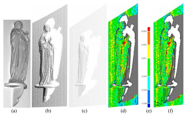
Fig. 7. Example "The Virgin Mary". (a) Intensity image of the object, (b) template surface, (c) search surface, (d) colored residuals between the fixed and transformed surfaces after the ICP method and (f) the LS3D surface matching method, (e) the residual bar in millimeter unit.
