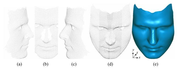
Fig. 5. Example "face". (a) Left-search surface, (b) center-template surface, (c) right-search surface, (d) obtained 3D point cloud after LS3D surface matching, (e) shaded view of the final composite surface.
