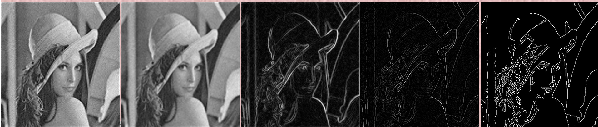
Original Image, Presmoothed Image, Gradient Image, Non-maximum Suppressed Image, Final Result
