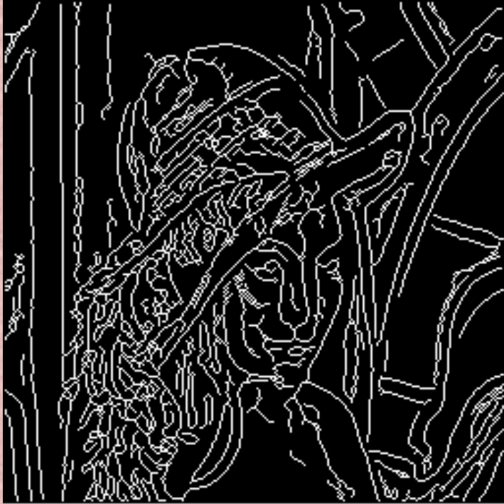
Scale space combination 2-D Canny edge model
