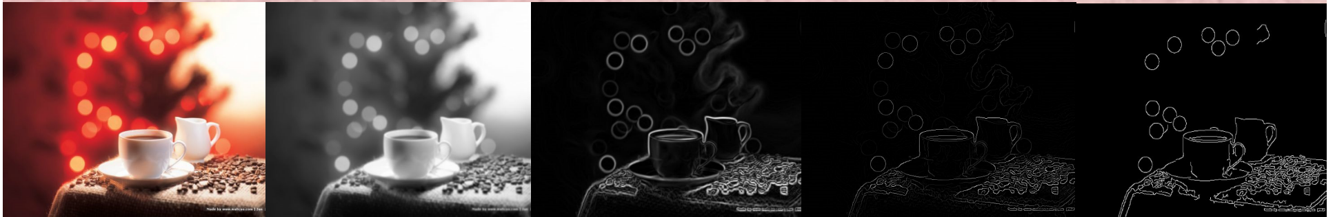
Original Image, Presmoothed Image, Gradient Image, Non-maximum Suppressed Image, Final Result
