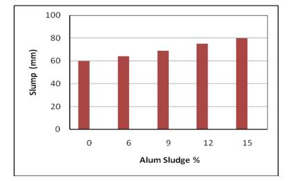
Figure 5 Effect of alum sludge on the slump
