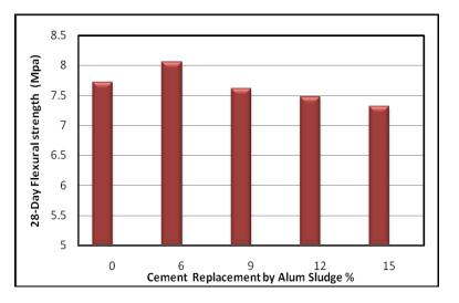
Figure 9 The effect of AS on flexural strength
