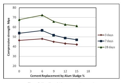
Figure 7 The effect of AS on compressive strength
