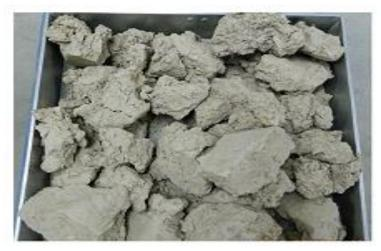
Figure 3 Alum sludge oven-dried at 110 °C
