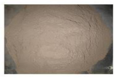
Figure 4 Ground alum sludge
