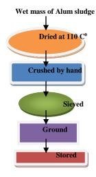
Figure 2 Schematic flow diagram of the preparation of the alum sludge sample
