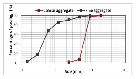
Figure 1 Grading curves of aggregates
