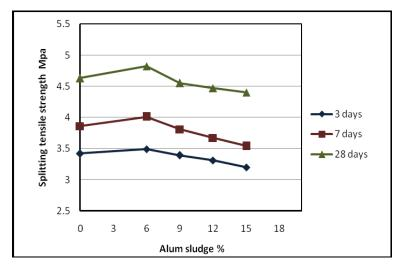
Figure 8 The effect of AS on splitting tensile strength
