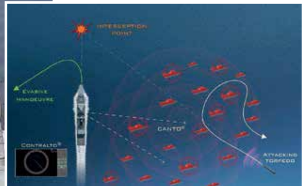
Main picture: C-Guard live firing from the frigate HDMS Iver Huitfeldt. Below: CANTO acoustic countermeasures concept of operations
