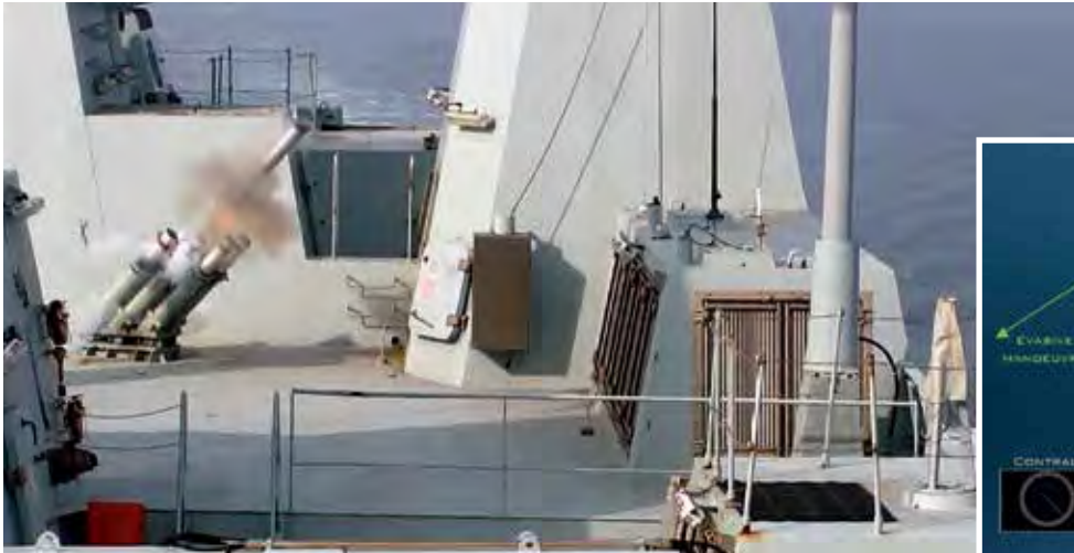
Main picture: C-Guard live firing from the frigate HDMS Iver Huitfeldt. Below: CANTO acoustic countermeasures concept of operations
