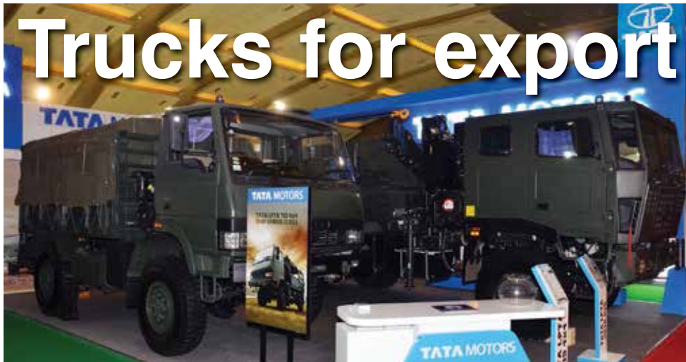
Tata Motors LPTA 715 (4x4) General Service truck (left) and the LPTA 2038 (6x6) high mobility vehicle
