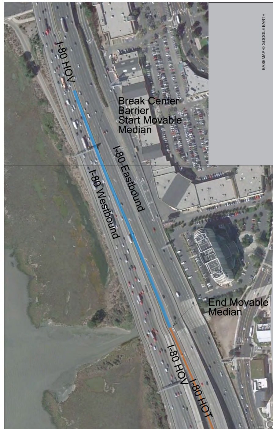
Figure 14: I-80 Contraflow Access
