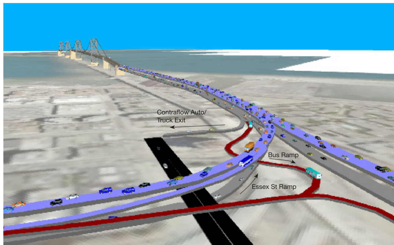
Figure 20: San Francisco Contraflow Lane Exit Option B
