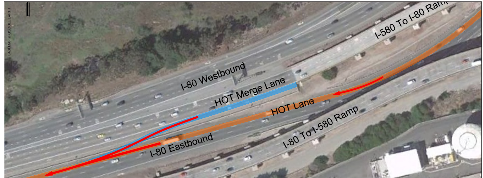
Figure 15: I-580 Contraflow Access
